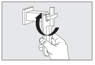
10 - Make sure the lever position is facing downward (6 o´clock position).
