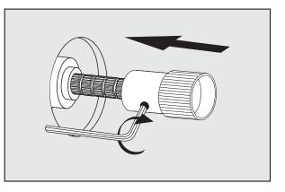
6 - After the connector is in place, remount the brass extension tube back onto the valve.
