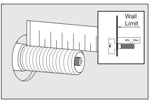
3 - *If the dimension exceeds the 1" "maximum" distance,* you must cut the brass extension tube and valve stem together as shown in the picture.
