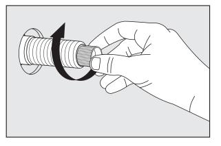
8- Slide the escutcheon onto the valve assembly. Slide the handle assembly onto the valve with the handle in the desired off position. Hold the handle in place and tighten the assembly as shown in picture 9.
