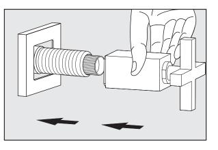
9 -Once the handle is placed and the posicion had been checked, use the provided wrench to adjust the escutcheon.
