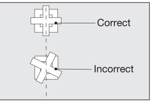
11- If you are unable to achieve the proper position, remove the handle and escutcheon from the valve, loosen the allen screw on the connector and remove it from the valve stem. Reposition the connector on the valve stem one nocht to the right or left, as needed to position your handle correctly. Tighten the connector and re-install the escutcheon and handle assembly.
