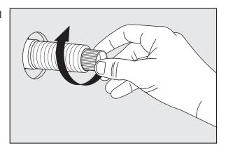
8- Slide the escutcheon onto the valve assembly. Slide the handle assembly onto the valve with the handle in the desired off position. Hold the handle in place and tighten the assembly by threading the escutcheon tube clockwise onto the connector.
