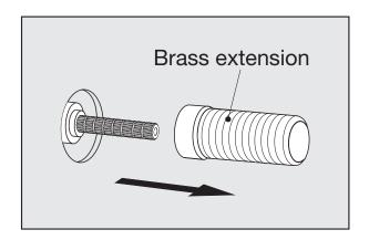
5- Place the connector on the stem and tighten with the provided allen wrench as shown in the picture.
