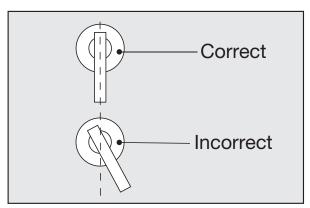
10- If you are unable to achieve the proper position, remove the handle and escutcheon from the valve, loosen the allen screw on the connector and remove it from the valve stem. Reposition the connector on the valve stem one nocht to the right or left, as needed to position your handle correctly. Tighten the connector and reinstall the escutcheon and handle assembly.
