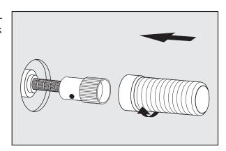
7 - Turn the connector clockwise until it stops. This is the "OFF" position.
