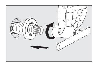
9 - Make sure the lever position is facing downward (6 o'clock position).
