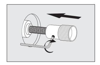
6 - After the connector is in place, remount the brass extension tube back onto the valve.
