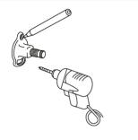
1\_Using the support (in the position the figure shows), mark the place where you will drill the first hole to mount the accessory.
