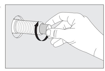
8- Place the handle by threading it's body on the brass extension.
