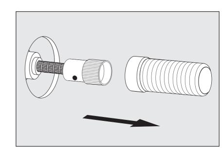
12- Remove, rotate, and reinstall the connector. And restart since point 6.
