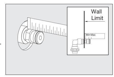
15 - To install the spout place it on the spout connector (is not necesary to thread it). Make sure the spout matches paralely with the horizontal and vertical lines wich were used to place all the pieces of the FV203/59.0 set.
