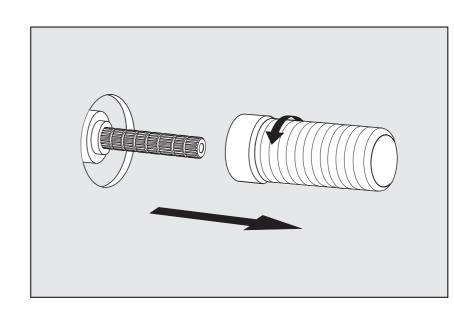
5- Place the connector and tight it with provided small allen wrench as shown in the picture.
