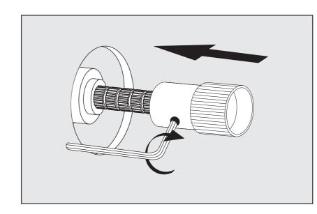
6 - After tighting the connector, place the brass extension.
