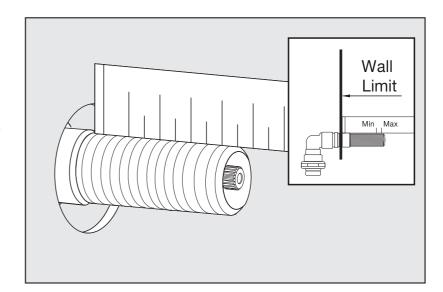
3 - <u>If the measured distance exceeds the "max" value</u> it's necesary to trim brass extension and valve stem (toghether).
