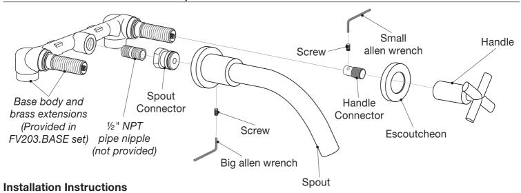
1- Make sure to place the valve with supply inlets pointed downward. The brass extension is already threaded onto the FV203.BASE body. It can be removed and trimmed using a saw along the provided groove, if necessary.
