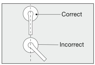
10- If you are unable to achieve the proper position, remove the handle and escutcheon from the valve, and remove it from the valve stem. Reposition the connector on the valve stem one nocht to the right or left, as needed to position your handle correctly. Tighten the connector and re-install the escutcheon and handle assembly.
