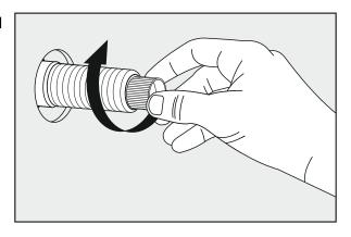
8- Slide the handle onto the valve assembly in the desired off position. Hold the handle in place and tighten the assembly by threading the escutcheon tube clockwise onto the connector.
