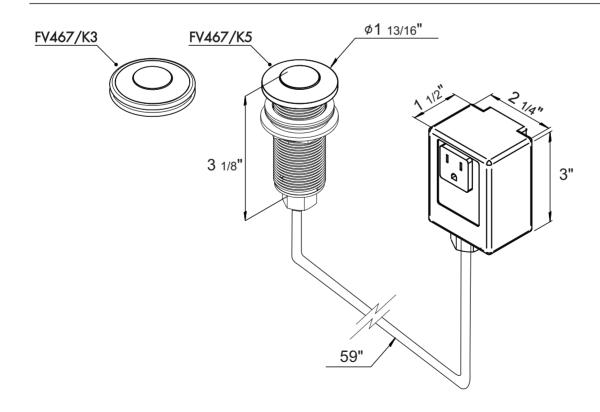
Connect tubing to bottom of unit.
